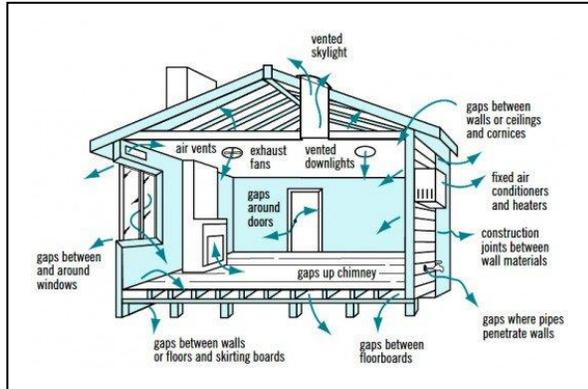
Blower Door equipment is utilized to conduct objective testing of the building envelope for air tightness. This comprehensive test confirms proper build practises during construction. Normally there would be 2 blower door tests completed during the build process. The first test is run when the building envelope including windows, and doors and there is no exterior or drywall finishes installed. This provides the
